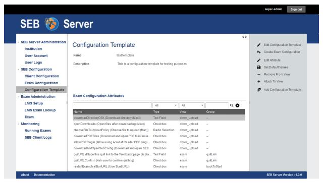
The type of the attribute defines the input field type and cannot be changed in any way. The view defines the tab on which the settings attribute is placed. And the group defines the named group where a settings attribute belongs to.
