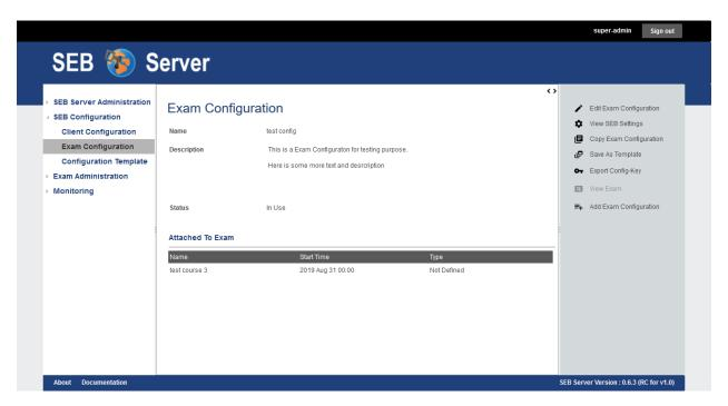
An exam configuration has a general settings part (like other domain objects has within SEB Server) that defines the name, description and status of the exam configuration that are used to maintain the exam configurations SEB Server internally. And a exam configuration has, separated from the general settings, the SEB settings that contains most of the SEB setting attributes as they are provided by the SEB.
