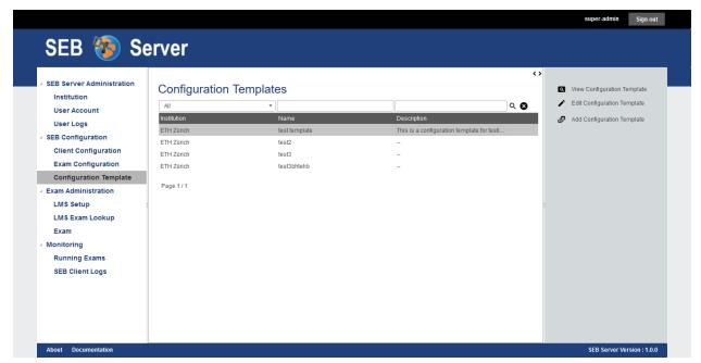
To create a new exam configuration template use the "Add Configuration Template" action from the right action pane. You will see the creation form with a name and description for the new template. At least a unique name is mandatory and the description is optional.
