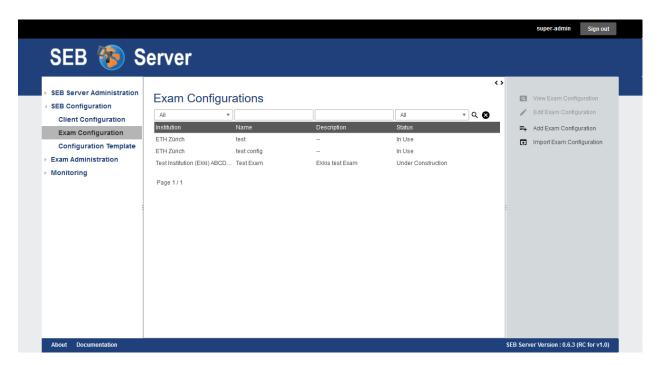
To view details of a specific exam configuration either double-click on a list entry or select a list entry and use the "View Exam Configuration" action from the right action pane. In the detail view all general settings are shown and also a list of exams that uses this exam configuration. In the current version of SEB Server, an exam configuration can only be assigned to one exam.
