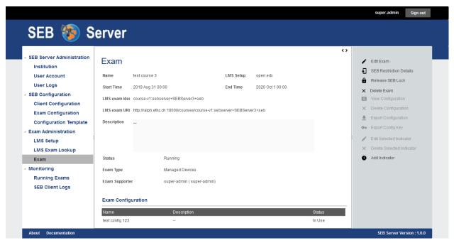
Use the "Apply SEB Lock" on an exam that has not already locked the course for SEB on the LMS to do apply the restriction and lock the course or quiz for SEB access only. This will call the SEB course restriction API on the LMS and will send all information to lock the course on the LMS. On an exam where the restriction lock is already in place, use the "Release SEB Lock" action to remove the restriction in the LMS and unlock the course.
